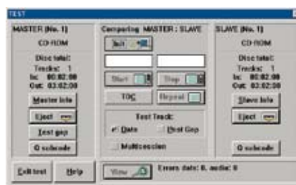
Compare: Compares Master-CD to stamper or replica up to 40x Speed Compares Lead-In, Lead-Out Postgap, Q-Subcode, ISRC; Data
